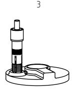
screw with bushing by hand or with manual installation tool at 0,25–0,70 mm under the edge of the surface
